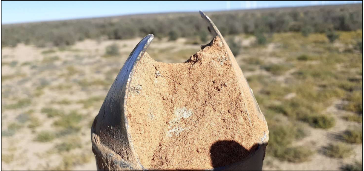
Figure 9: Soil sample taken within one of the indicated non-FEPA wetland depressions that exhibited salt precipitates.
