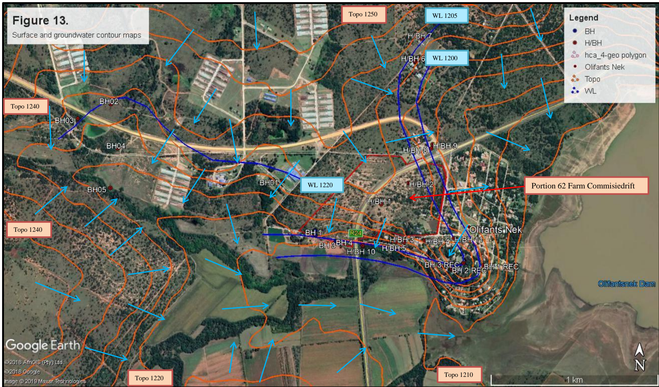
Figure 13: Contour map showing 5 meter interval surface contours with 5 meter groundwater contours with groundwater flow directions (blue arrows)
