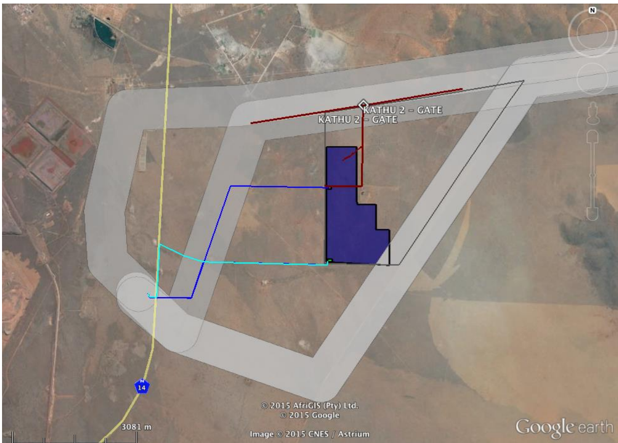
Figure 15: Map of the proposed Eskom routing corridors for the 66Kv to 132Kv network upgrade in relation to the proposed PV site.
