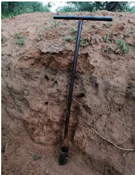
Glencoe soil form. Orthic A-horizon overlying a Yellow-brown Apedal B-horizon overlying a Hard Plinthic B.
