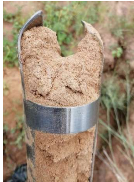
Weak structure overlying a low permeable Hard Plinthic layer with Fe- and Mn-oxides.
