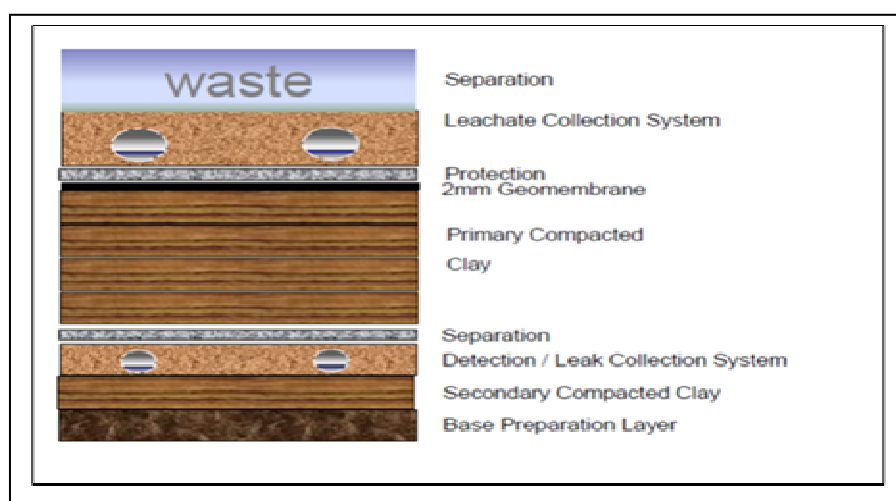
Figure 1: The different lining layers of the construction of the coal stock yard.
