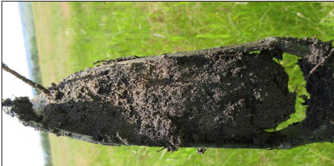
Figure 18: Hydric soils included a Sandy Clay Loam soil form associated with the wetland areas.
