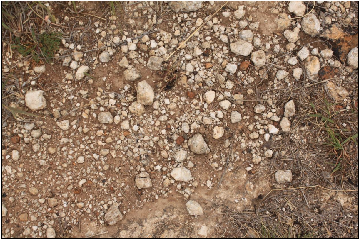
Figure 8: Coega soils within the grid assessment corridor with nodules of hard carbonate visible on the surface
