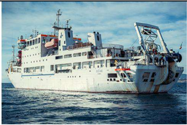
Figure 2.2 RV Teliri Cable Laying Vessel
