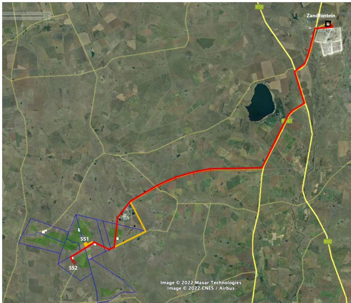
Figure 2: Google image of the Impumelelo gridline site. SS1 & SS2 = substations 1 & 2 at Impumelelo. Orange gridline starts at SS1 and the red gridline at SS2.
