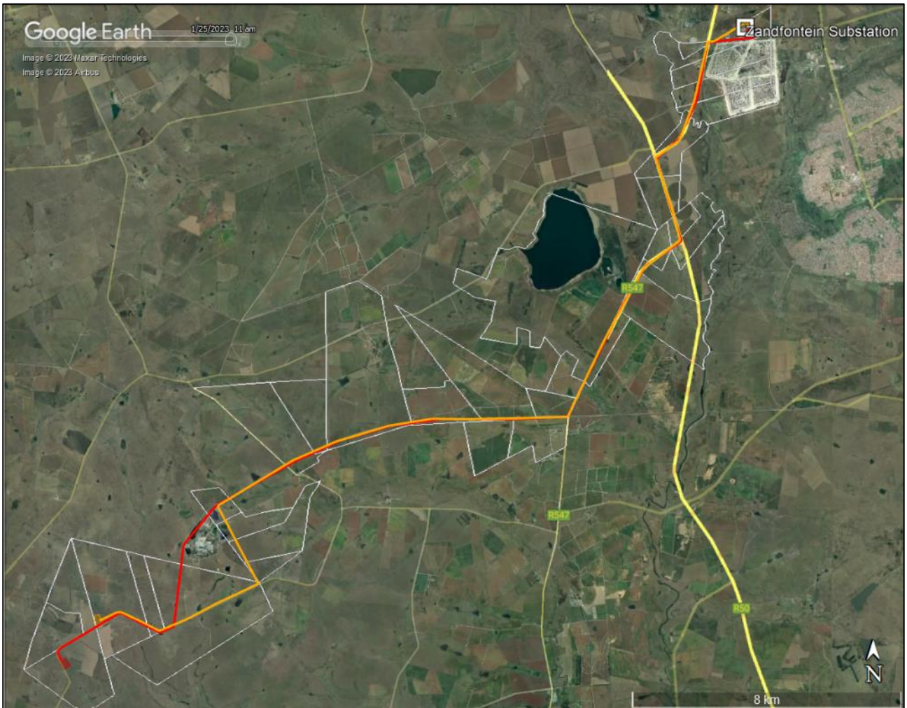
Figure 3: Proposed project layout. Orange block and line are the Alternative 1 substation and powerline, Red is Alternative 2).
