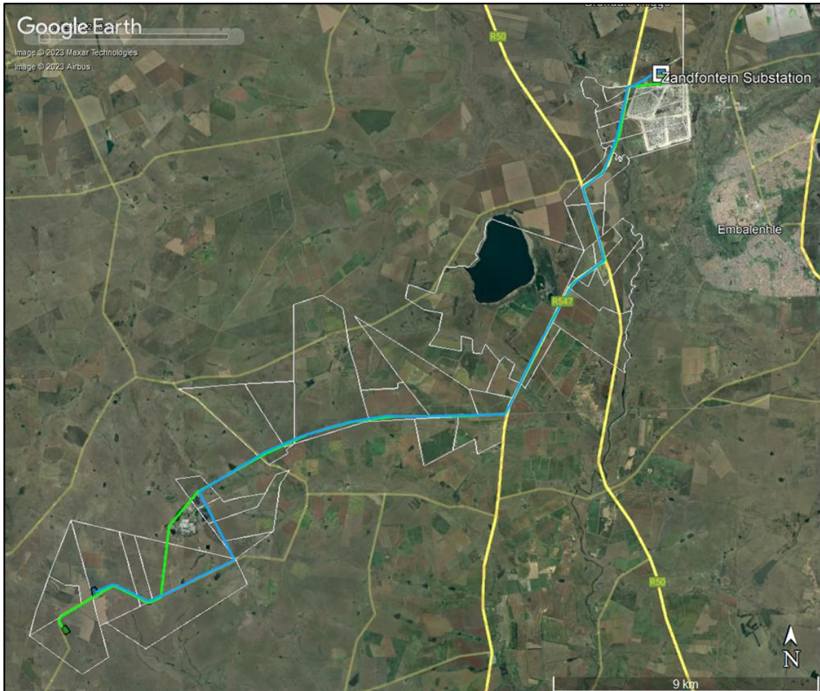
Figure 2: Impumelelo WEF grid route. Green block and line are the Alternative 1 substation and powerline, Blue is Alternative 2). Secunda is in the northeast and Greylingstad in the southwest of the sites.
