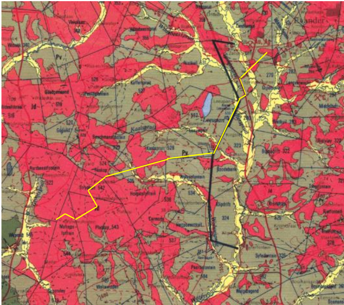
Figure 3: Geological map of the area around the Impumelelo WEF and proposed power lines. Yellow line is the proposed grid connection route. NB – western section with alternates all on dolerite. Abbreviations of the rock types are explained in Table 4. Map enlarged from the Geological Survey 1: 250 000 map 2628 East Rand.
