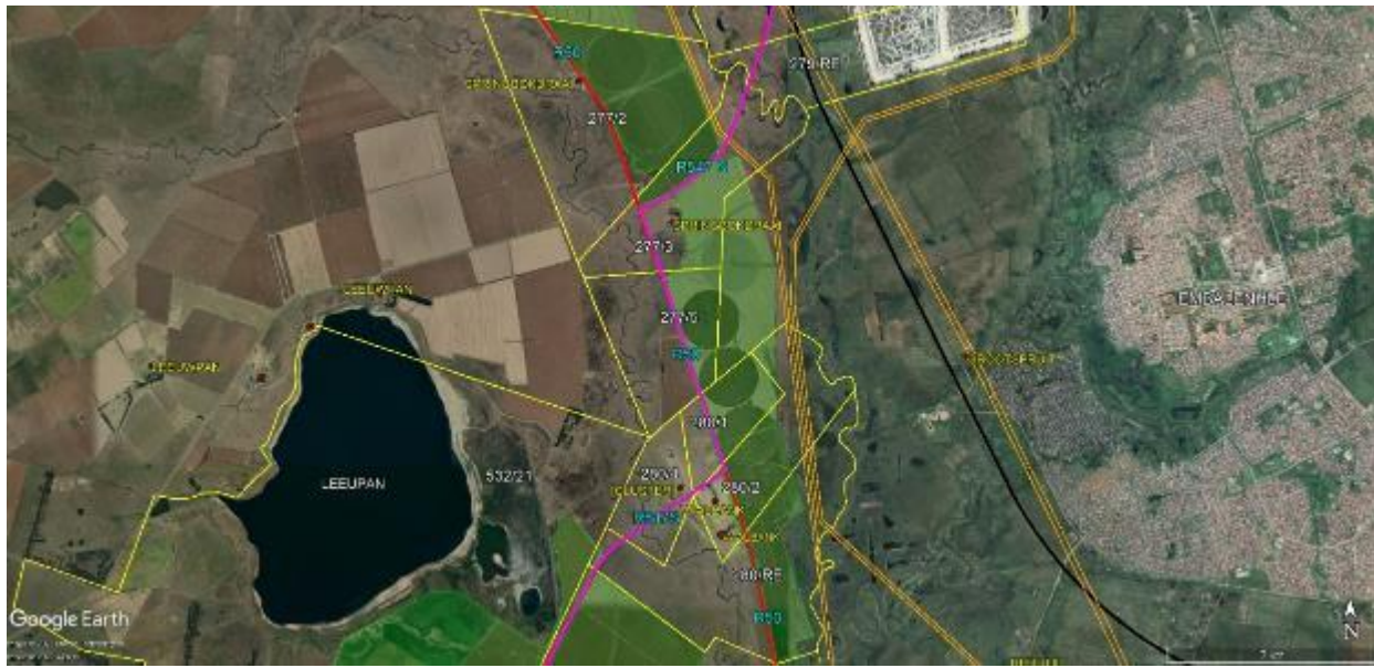
Figure 3.5: Overview of properties (yellow outlines) affected by Impumelelo grid connection proposal alignment portion along R50. The common alignment section is indicated in pink. Also indicated are local roads (red), coal conveyor belt corridors (black), existing overhead power lines (orange), and contiguous cropping areas on affected properties (green fill).
