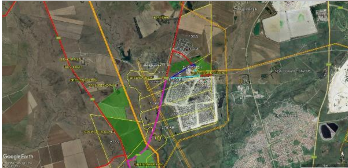
Figure 3.4: Overview of properties (yellow outlines) affected by Impumelelo grid connection proposal alignment portion from Brendan Village to 400 kV corridor. Alternative 1 alignment indicated in dark blue, Alternative 2 in light blue, and common alignment section in pink. Also indicated are local roads (red), coal conveyor belt corridors (black), existing overhead power lines (orange, 400 kV corridor in bold), and contiguous cropping areas on affected properties (green fill)
