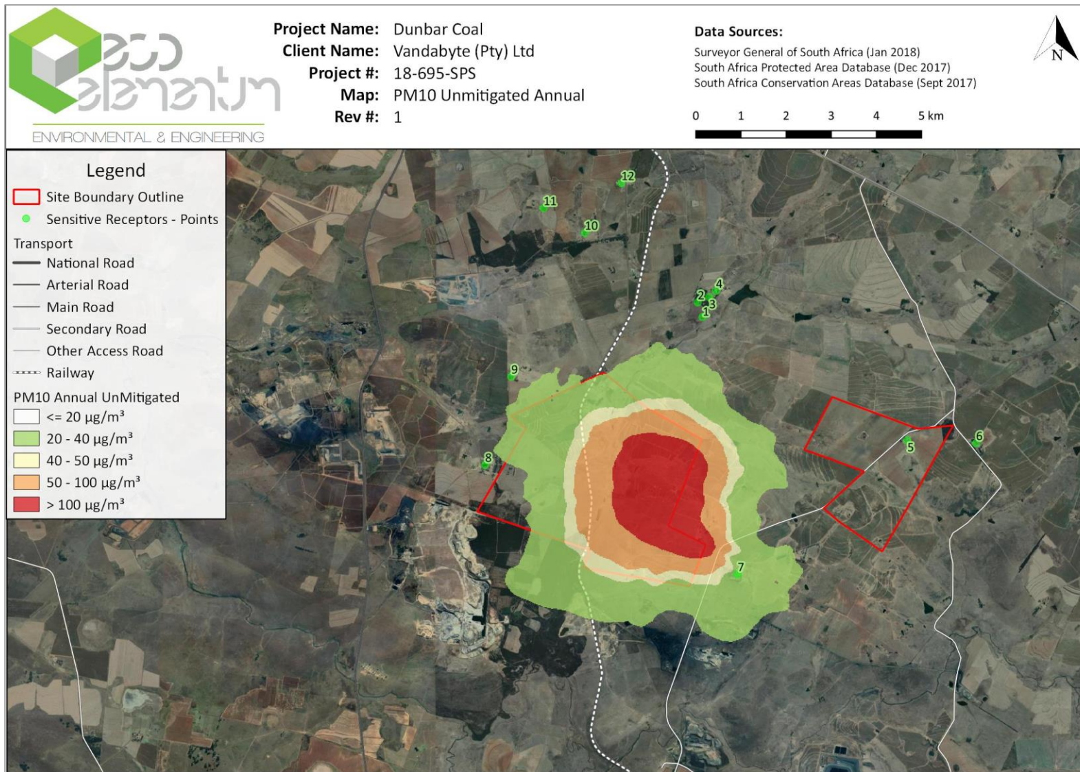
Figure 17: Predicted average annual concentrations for PM10 for the proposed Dunbar Coal project when unmitigated.
