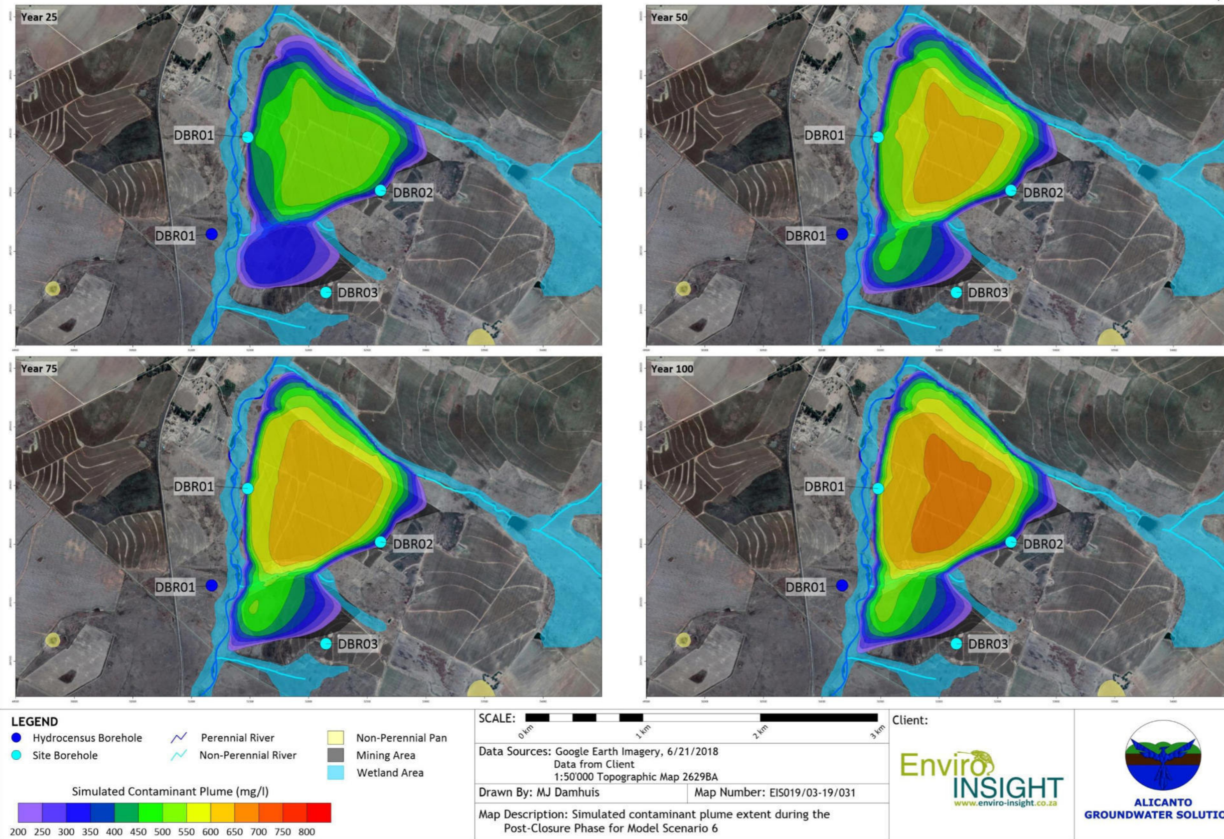
Figure 9.22: Simulated Contaminant Plume Extent (Post-Closure Phase) - Scenario 6
