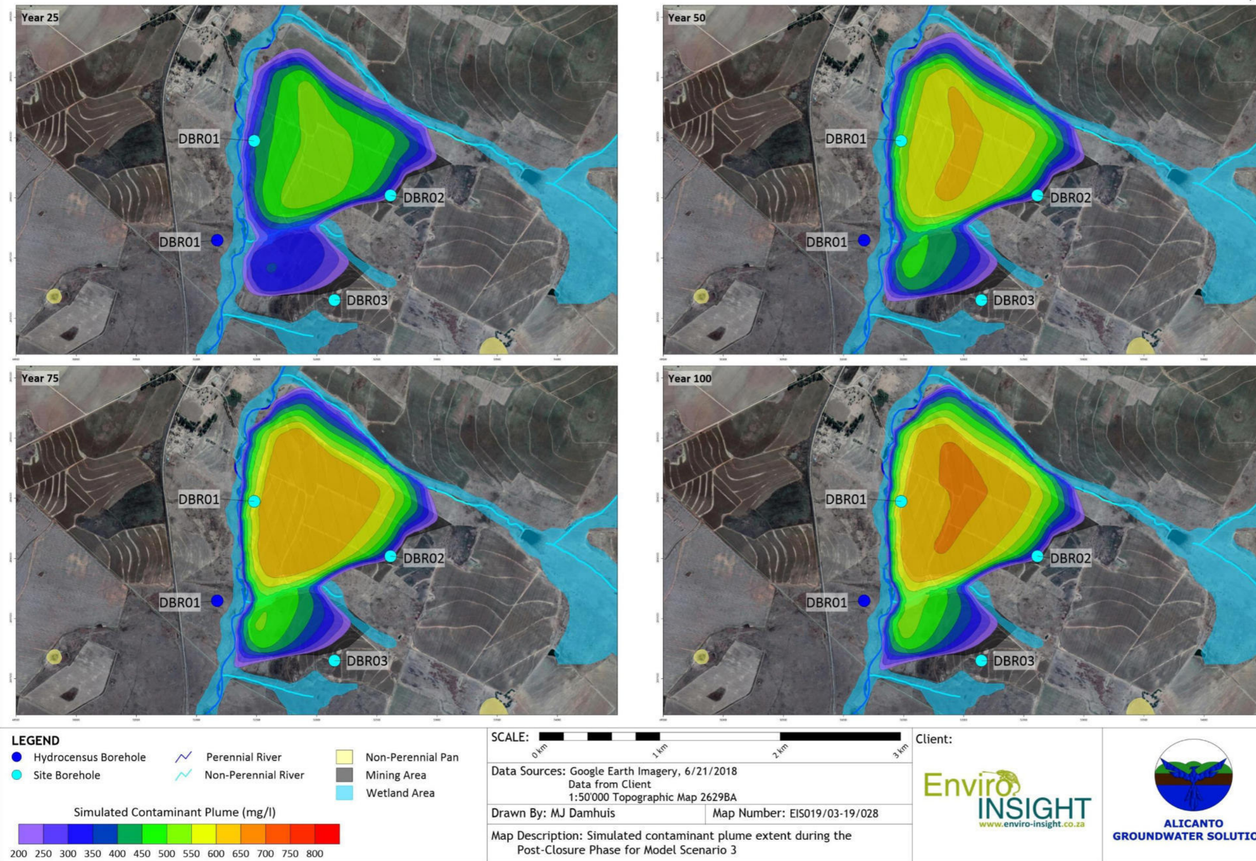
Figure 9.19: Simulated Contaminant Plume Extent (Post-Closure Phase) - Scenario 3
