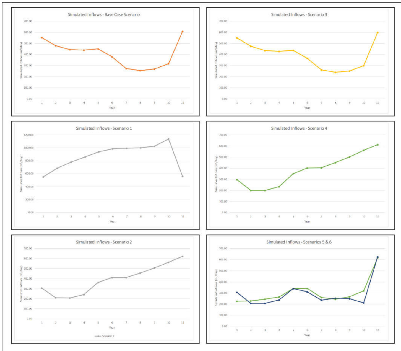
Figure 9.1: Simulated Inflows to Opencast 1 and Opencast 2 during the Operational Phase
