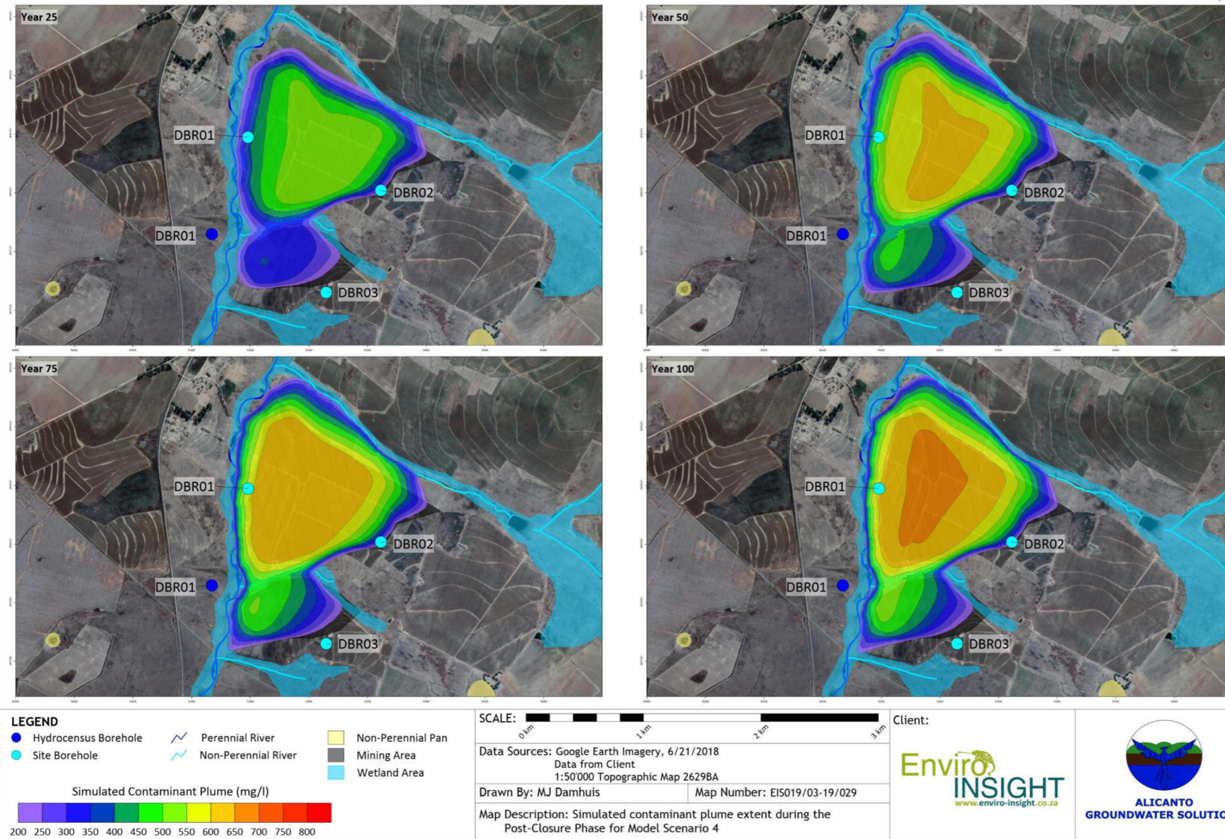
Figure 9.12: Simulated Contaminant Plume Extent (Operational Phase) - Scenario 4
