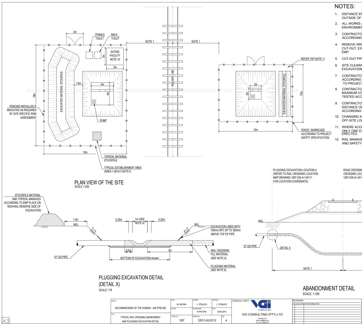
DISTANCE ENGINEERED TO ENSURE PLUGGING EXCAVATIONS ARE LOCATED OUTSIDE OF BOUNDARY OF RAIL RESERVE.
