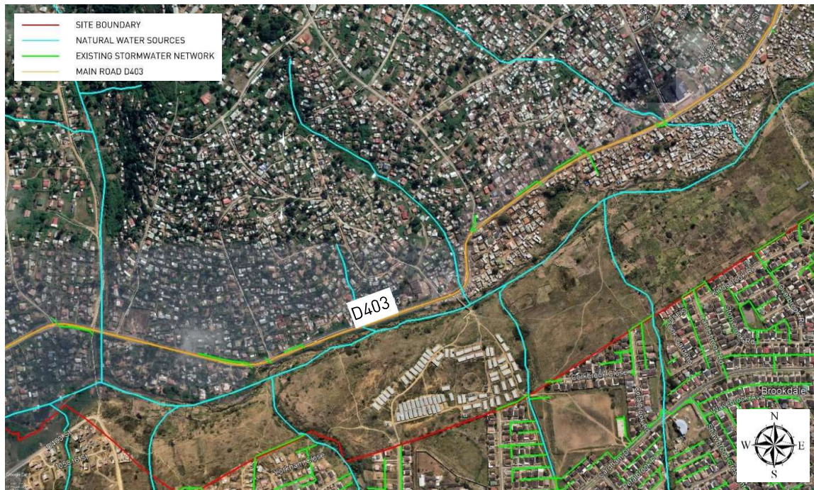
FIGURE 12: EXISTING STORMWATER SYSTEM ALONG D403
