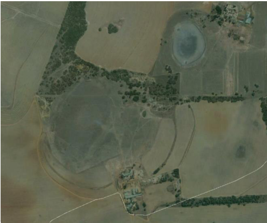
Figure 26 Pan system with two pans that are not connected to drainage features on the surface
