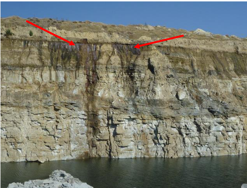
Figure 20 Opencast mine profile indicating a distinct flow path (arrow) beneath the soil profile
