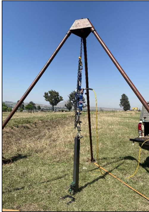
Figure 4: Vertical uplift test setup 1
