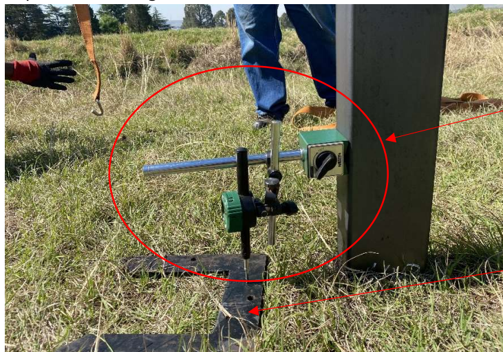
Figure 5: Dial gauge measuring setup
