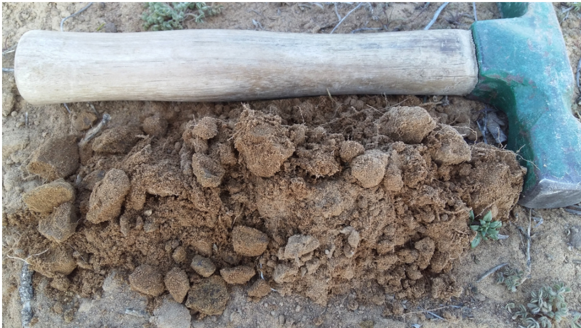
Figure 10 Photographic evidence of a shallow Bethesda form identified on site (the neocutanic subsoil horizon is limited in depth by fractured rock)
