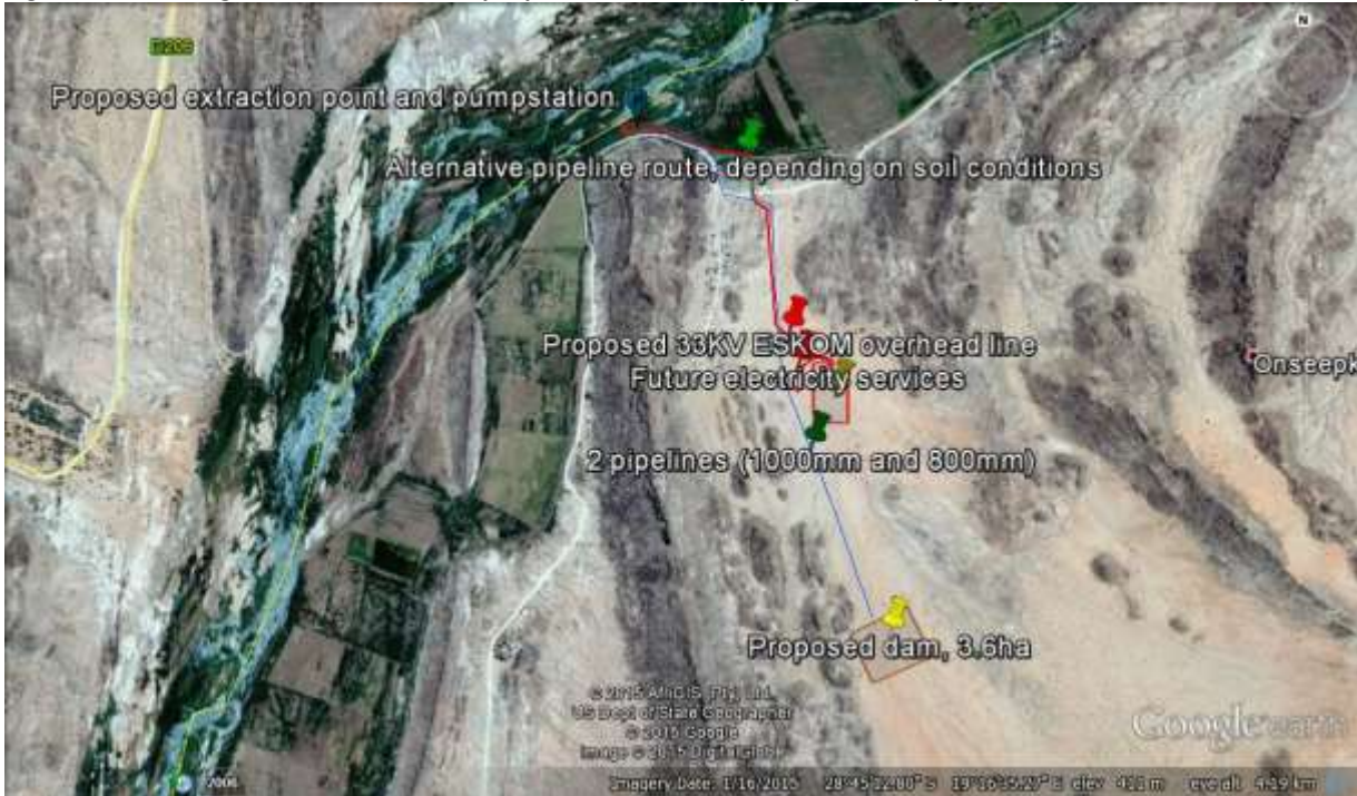
Figure 1: Showing the location of the proposed dam, SPV, pumpstation, pipeline and overhead cables
