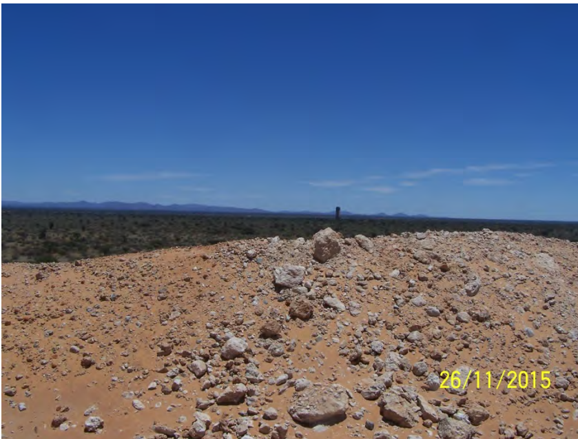
Figure B12: Calcrete heaps mixed with Kalahari sand at the top of Northern dump
