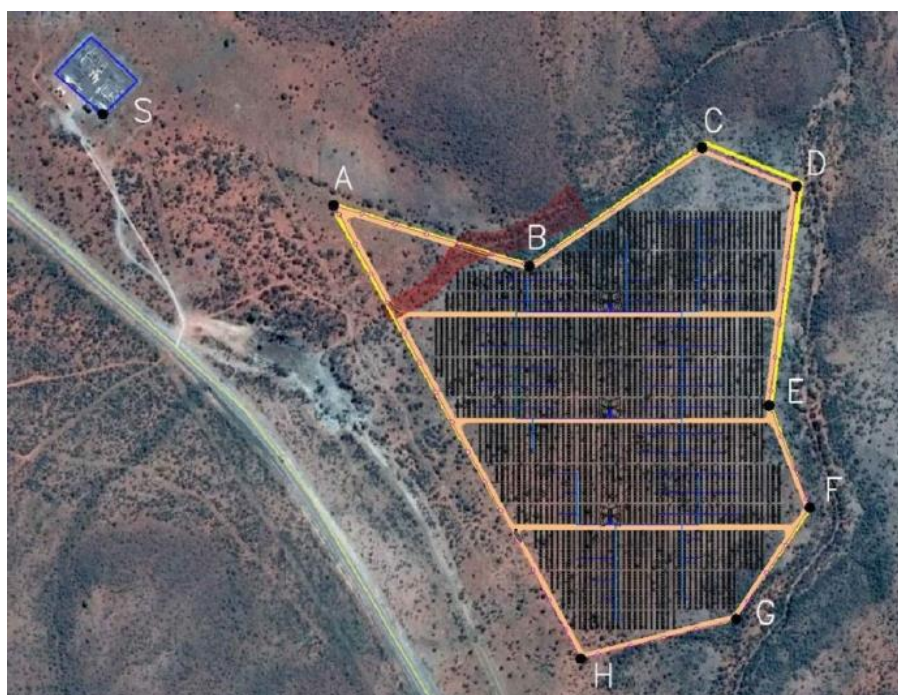
Sensitivity Map 1 – Red shaded area indicates 32m setback buffer zone between watercourse within the site and proposed layout area of the solar PV panels.
