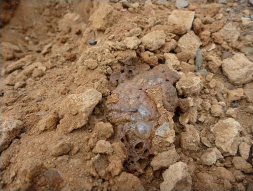
Figure 11 Effervescence of the soil with a 10% HCl solution indicating the presence of lime
