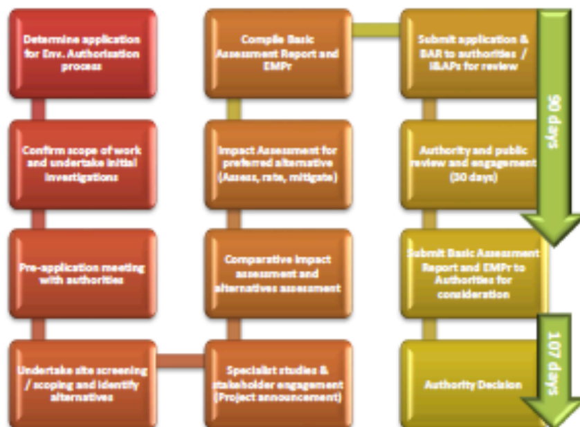
Figure 2: Process Flow Diagram for the steps required in a Basic Assessment Process
