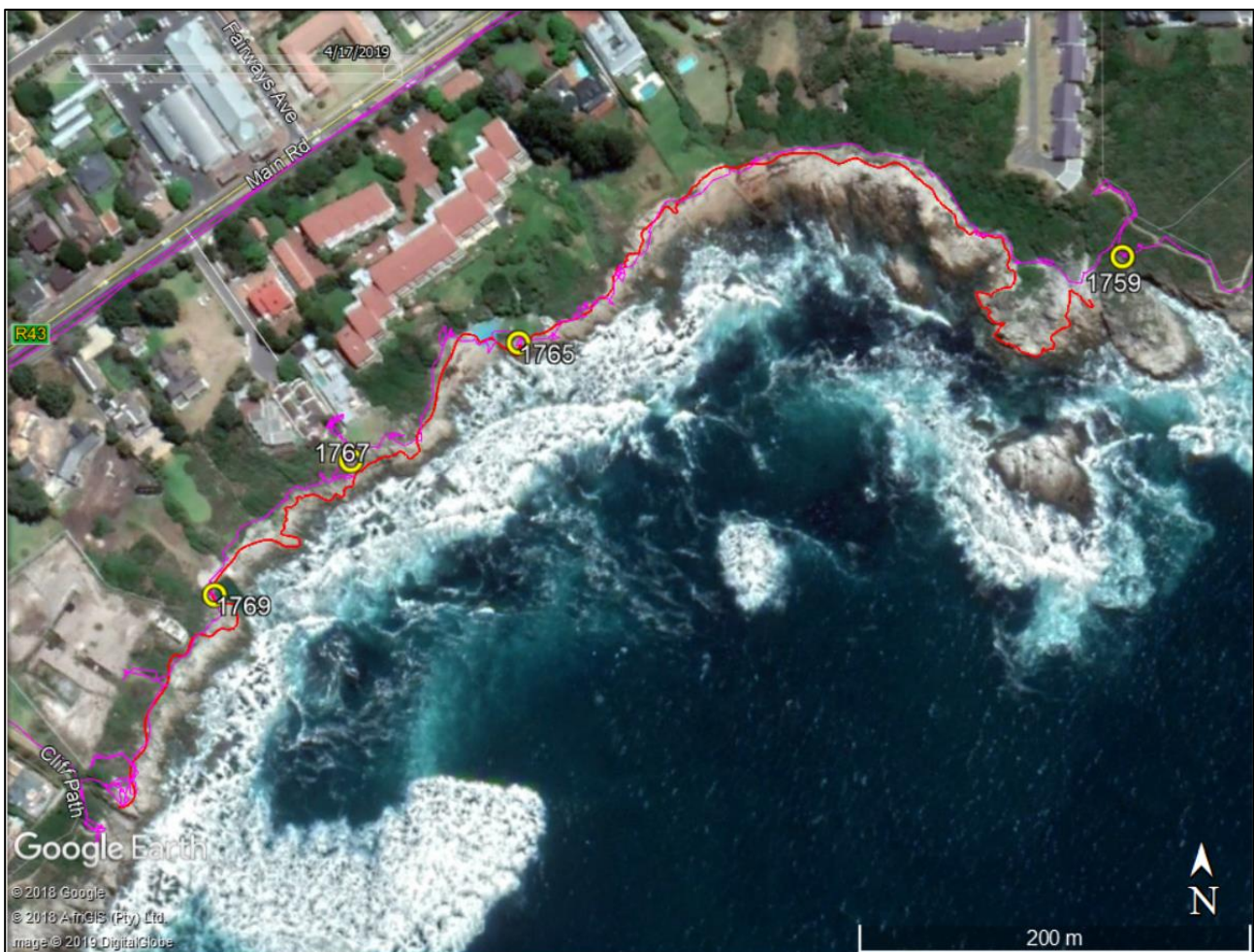
Aerial view of the study area showing the recently surveyed high water mark (red line; still to be approved by the Surveyor General), the survey tracks (purple line) and the waypoints mentioned in this application (numbered yellow symbols).
