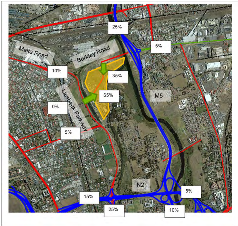
Figure 10: Distribution on Partially extended Road Network
