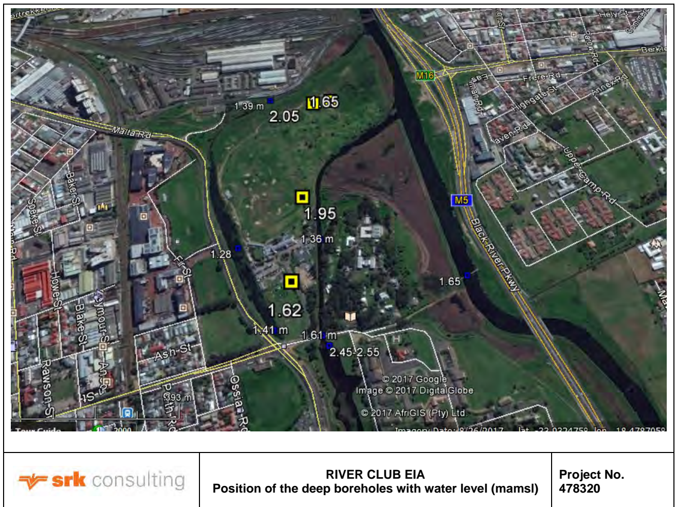
Figure 1: Positions and water levels of boreholes
