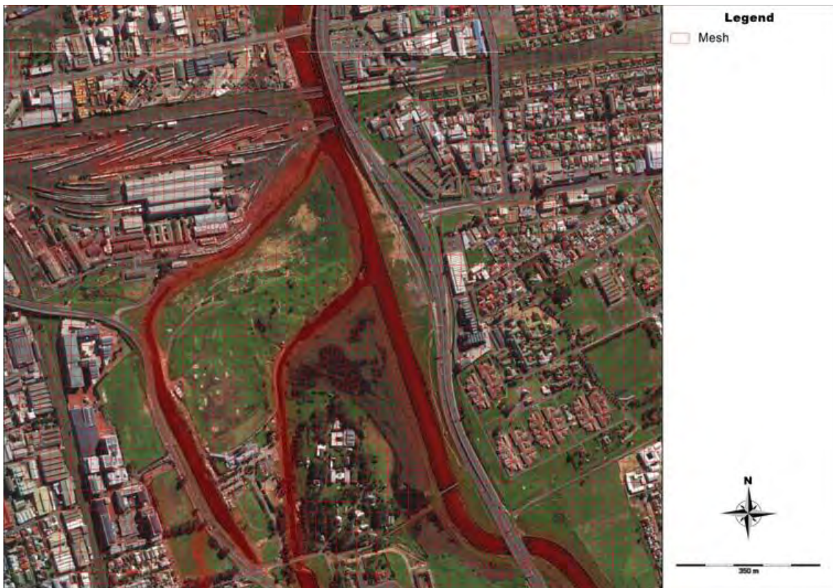
Figure 3-7 HEC-RAS 2D Mesh – showing varying resolutions
