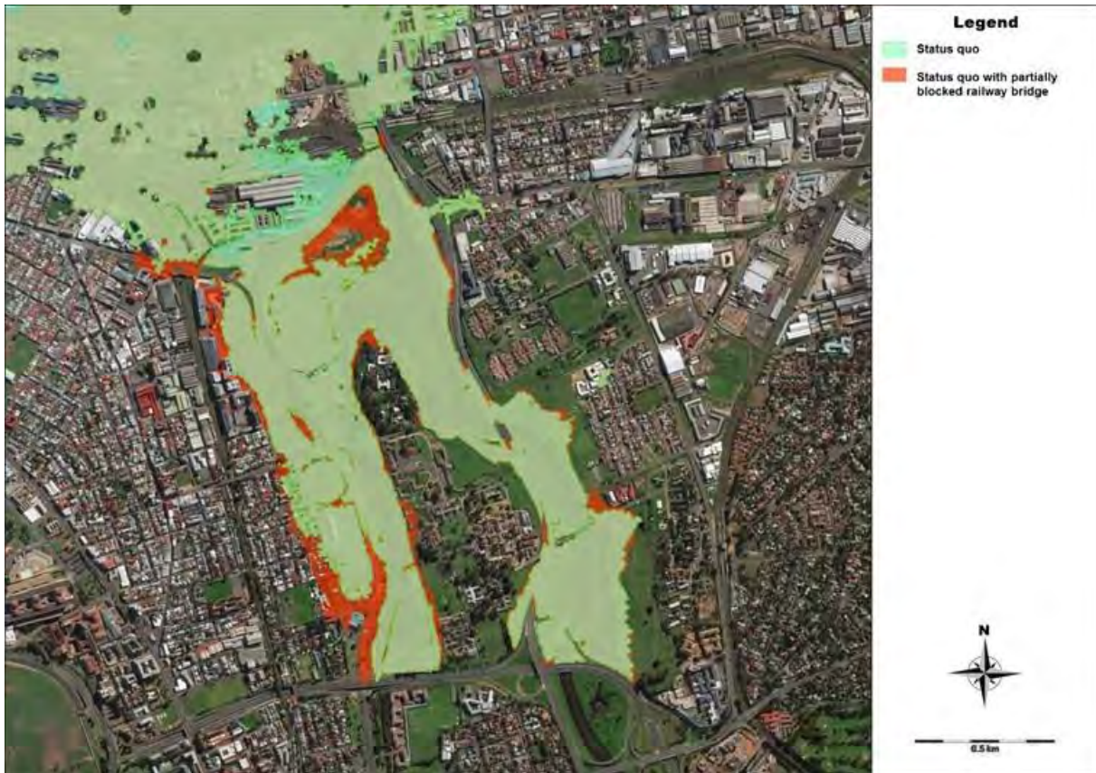
Figure 4-12 Impact of partially blocking the railway bridge immediately downstream of the River Club site
