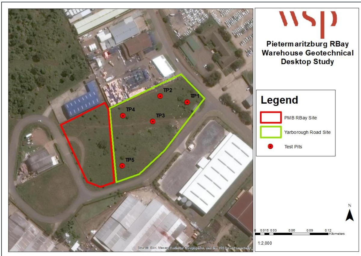
Figure 4-1 - Position of the test pits on the adjacent site
