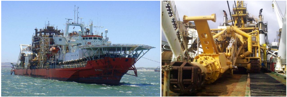
Figure 3-4: The MV Ya Toivo (left) and its MK2 seabed crawler (right).
