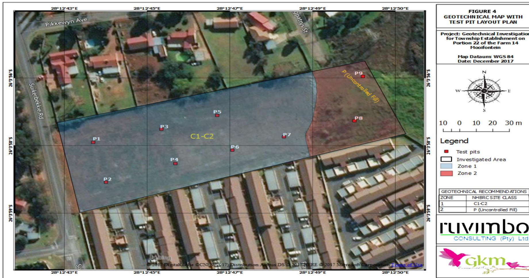
Figure 4: Test Pits Position and Geotechnical Zonation
