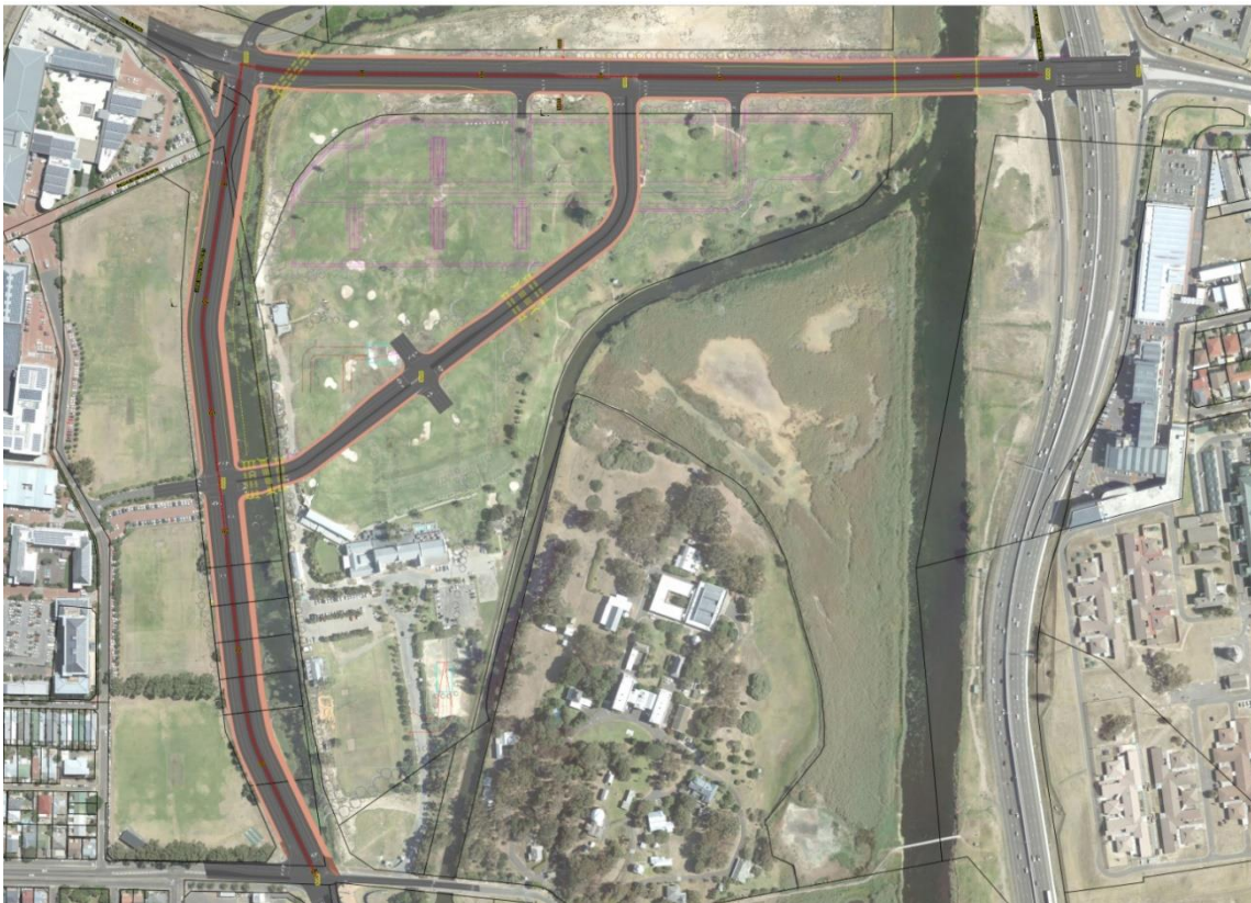
Figure 12: Proposed layout of the Berkley Road Extension and the proposed T-junction with Liesbeek Parkway (Aurecon in consultation with the City of Cape Town’s TDA) 18
