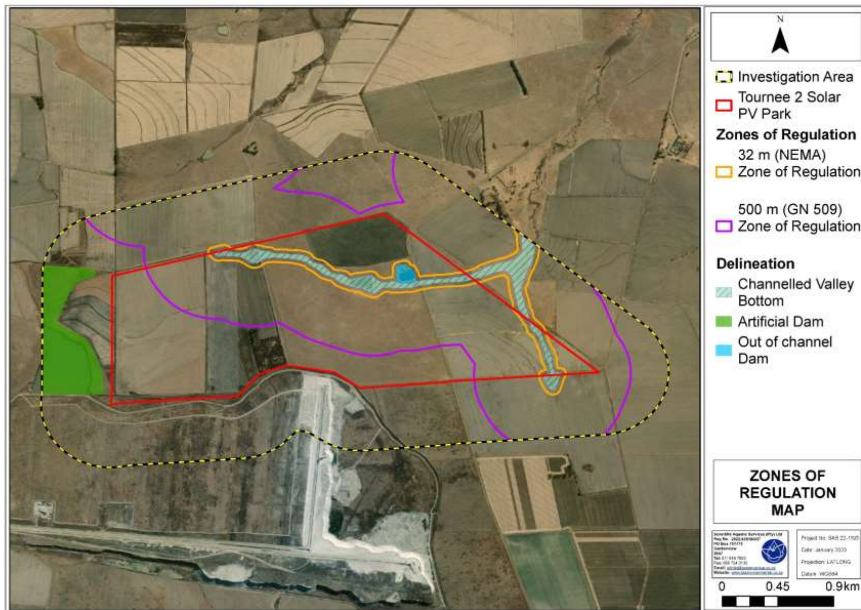
Figure 16: The applicable Zones of Regulation related to the proposed Tournee 2 Solar PV Park according to the GN 509 and NEMA.
