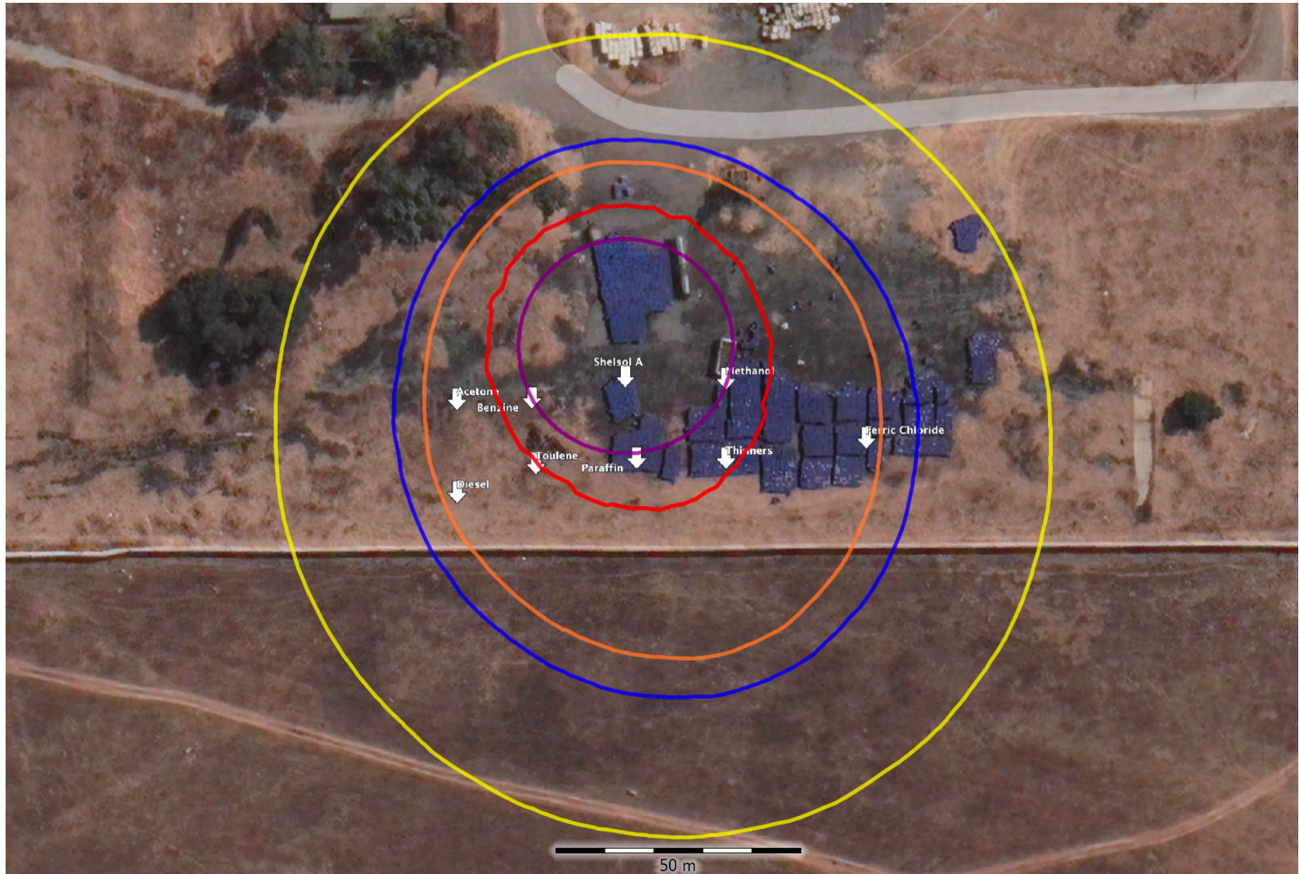
Pool Fire Consequences of a Catastrophic Failure at the Shellsol A Road Tanker
