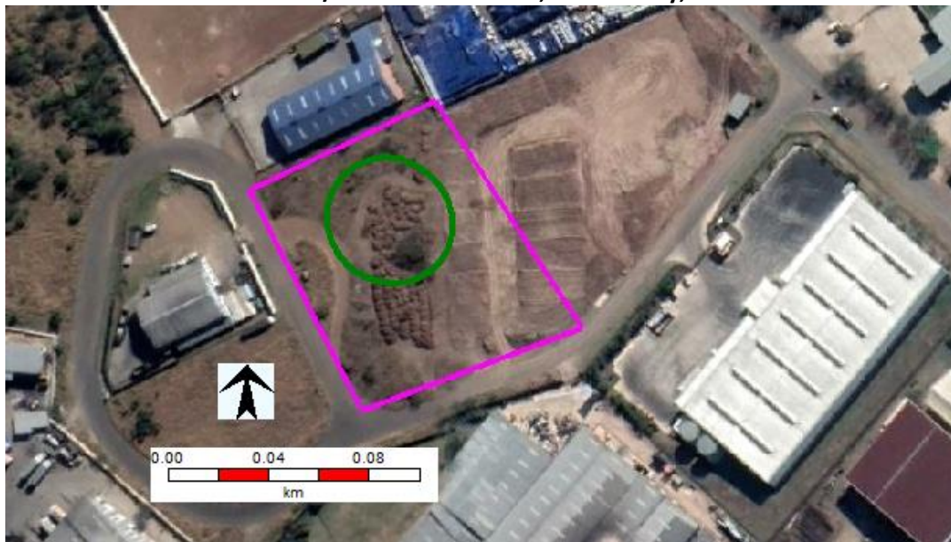
Figure 5.2.1.1 Radiation effects from a late pool fire resulting from the catastrophic rupture of one pallet with four drums of acetic acid
