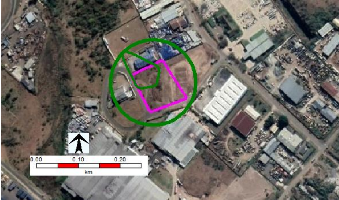
Figure 5.1.3.1 Lethality effect zone- catastrophic rupture of one pallet (4 drums) of 25% ammonium hydroxide solution by forklift while offloading(S9).
