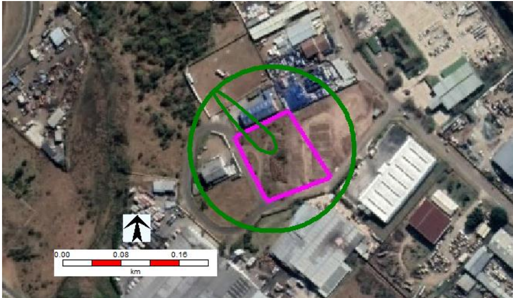
Figure 5.1.1.2 Lethality effect zone- catastrophic rupture of one drum of 33% hydrochloric acid by forklift while offloading(S1).
