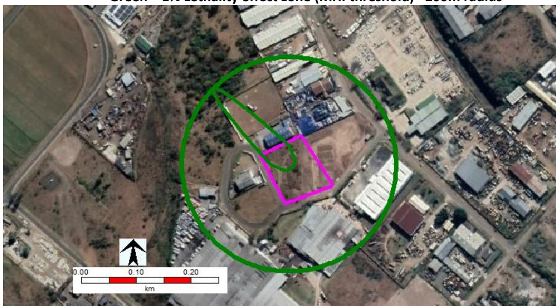
Figure 5.1.1.2 Lethality effect zone- catastrophic rupture of one pallet (4 drums) of 33% hydrochloric acid by forklift while offloading(S1).
