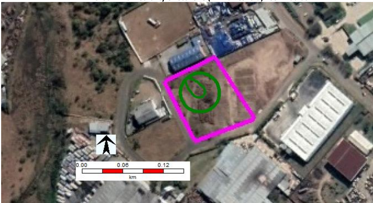
Figure 5.1.2.1 Lethality effect zone- catastrophic rupture of one pallet (4 drums) of nitric acid by forklift while offloading(S4).
