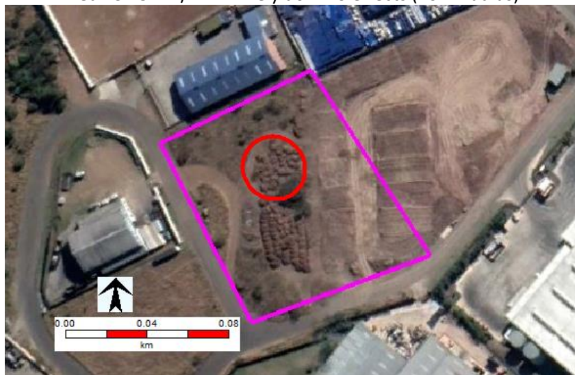
Figure 5.4.1 Potential domino effect zone - catastrophic rupture of acetic acid leading to a late pool fire, Red= 37.5 kW/m 2 – Likely domino effects (20 m radius)
