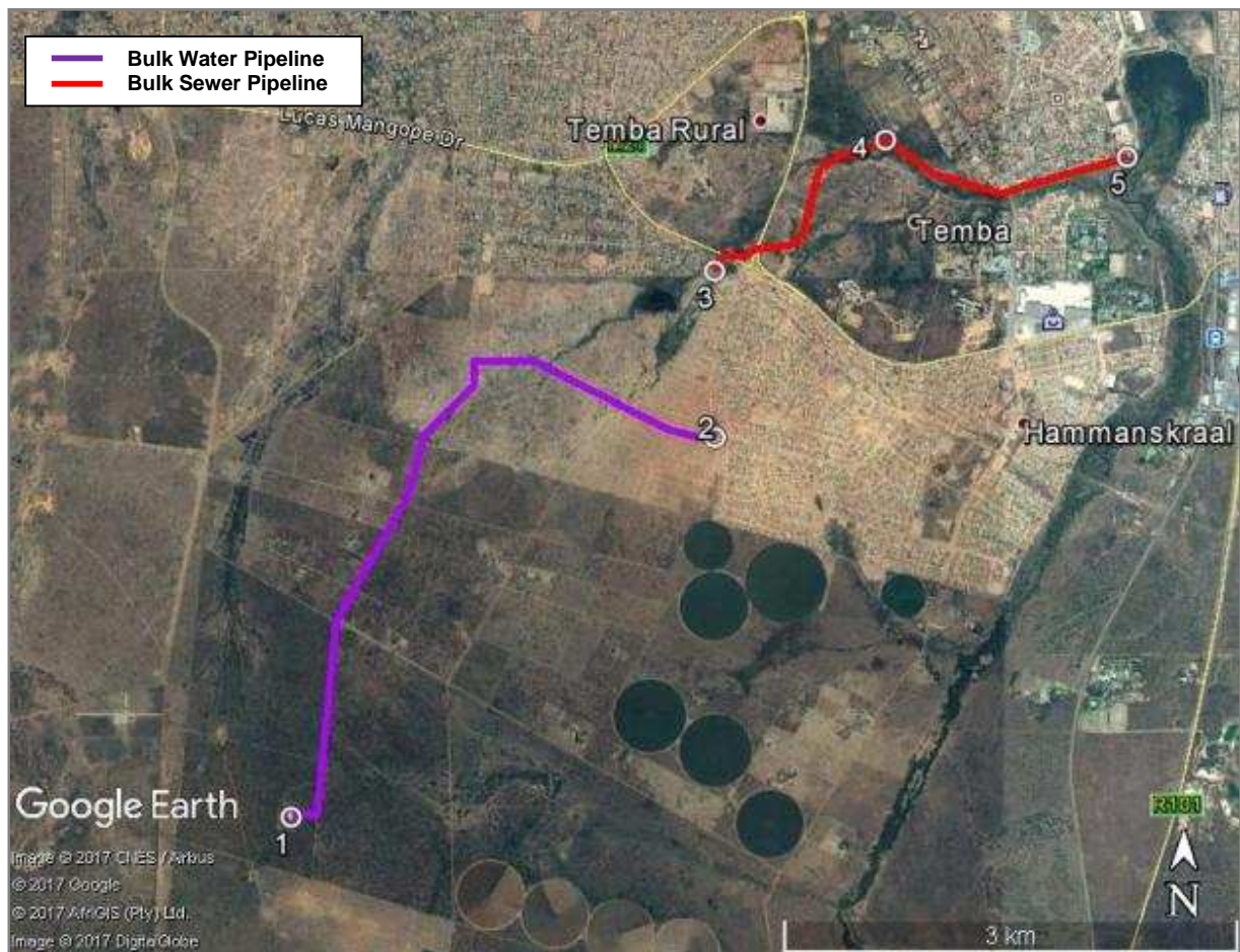
Figure 2: Proposed bulk water and sewer pipelines
