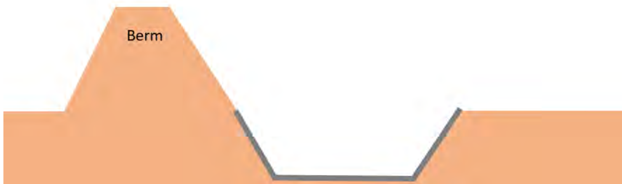
Figure 11: Perimeter channel cross-section schematic.
