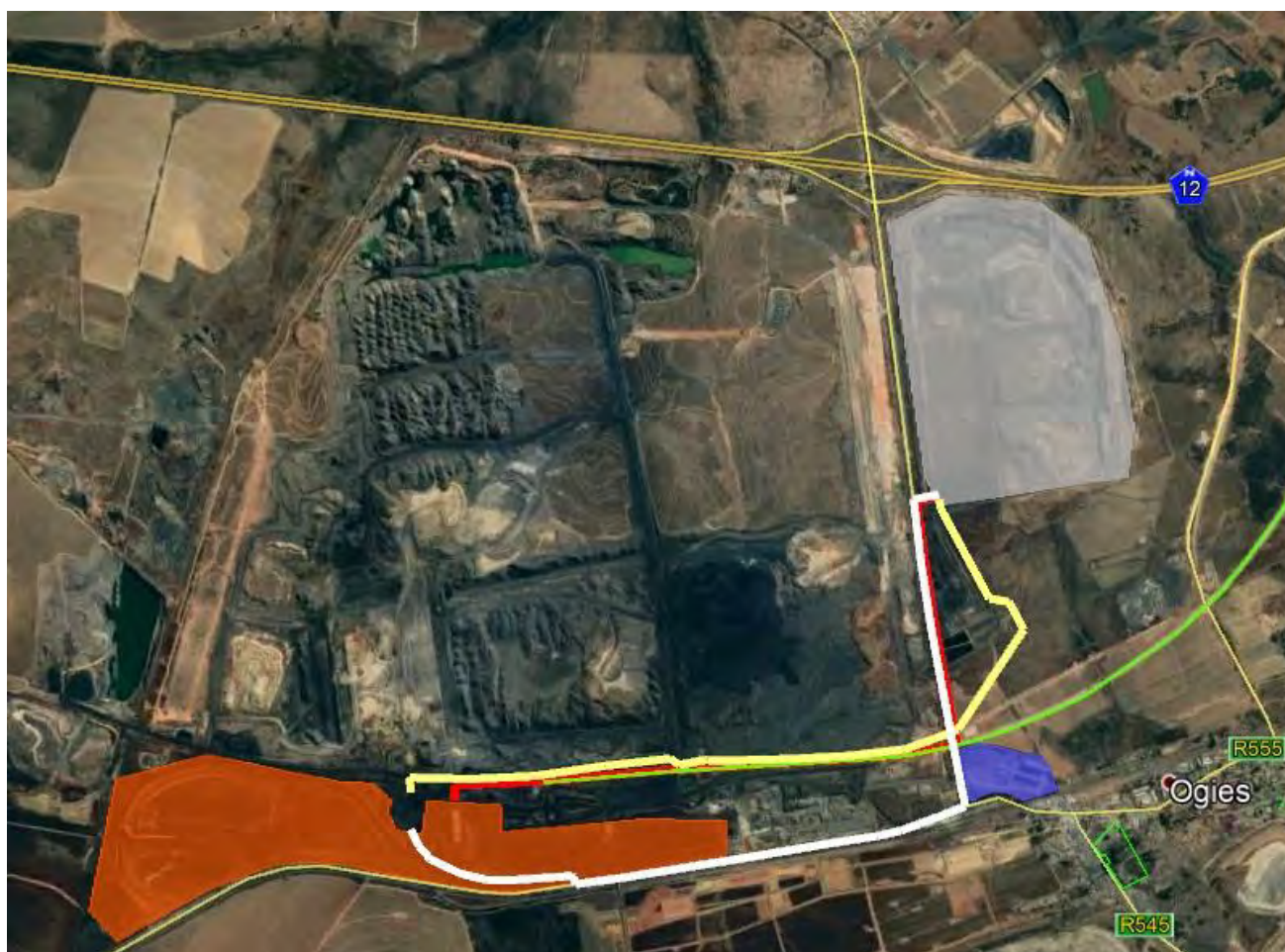
Figure 4: Map indicating conceptual alignment of proposed discard transport alternatives. A public road route in white, a proposed mine Road crossing the South 32 property in yellow and proposed new conveyor route in red. The alignment of an existing coal conveyor is indicated in green.
