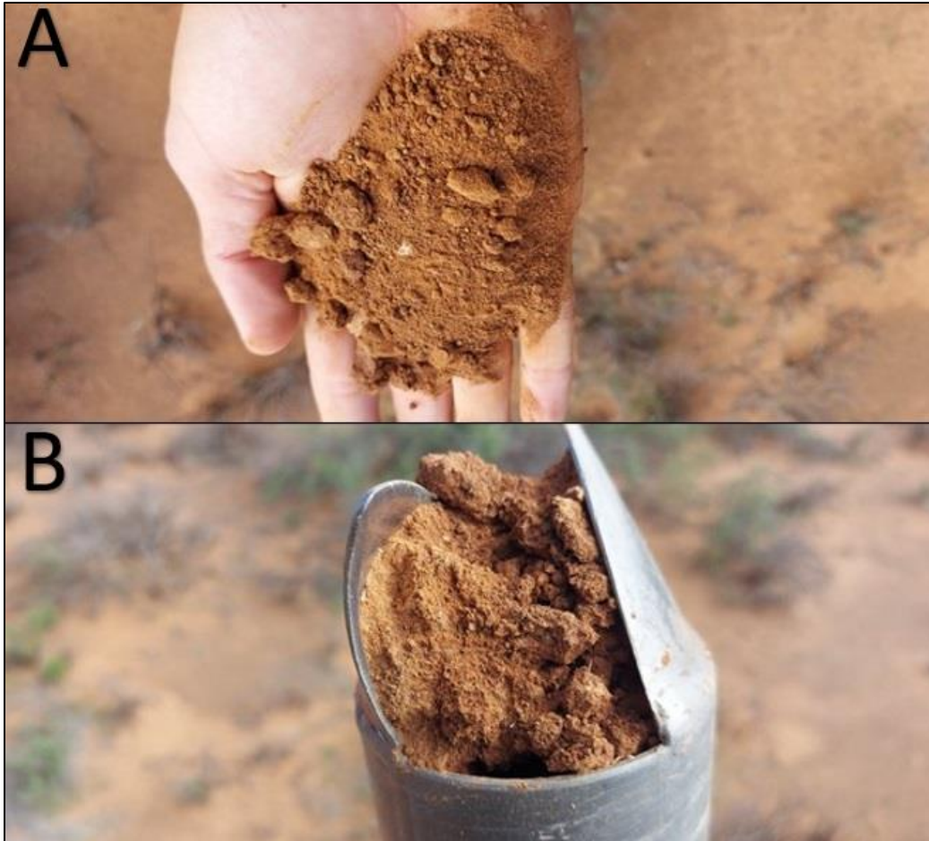
Figure 8-1 Examples of horizons associated with the Tubatse and Bethesda soil forms. A) Neocutanic horizon. B) Transition between neocutanic and lithic horizon
