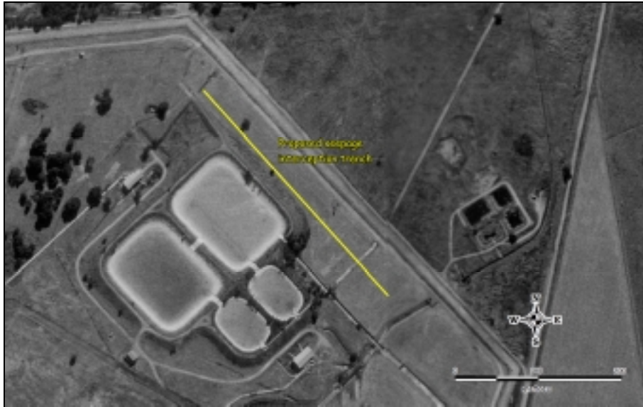
Figure 76. Position of proposed interception trench at the High Level Ash Water Return Dams.
