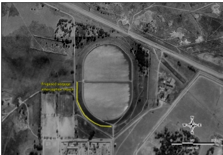
Figure 56. Possible location and orientation of a seepage interception trench on the western and south-western perimeter of the Raw Water Dam.
