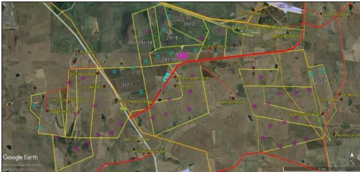
Figure 3.6: Turbine and substation locations indicated as acceptable (pink) and unacceptable (blue) by the relevant land owners.
