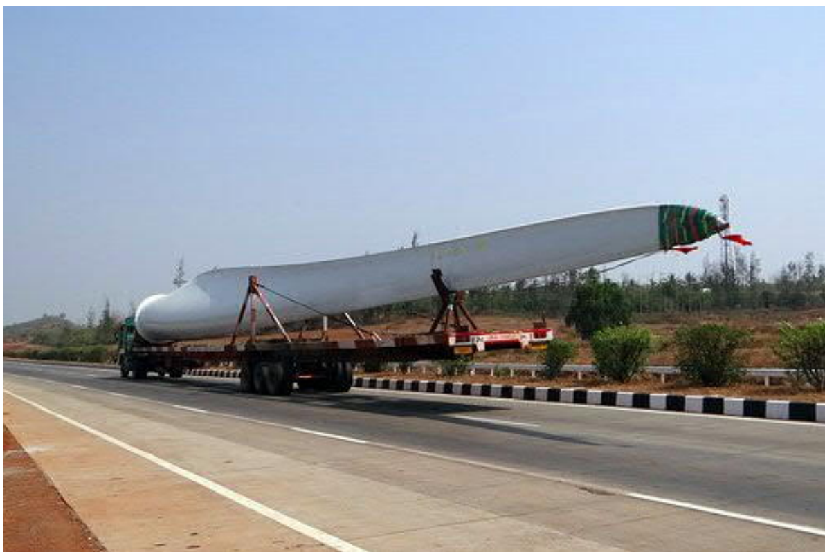
Figure 4-4: Blade transport (Froese, 2019)
