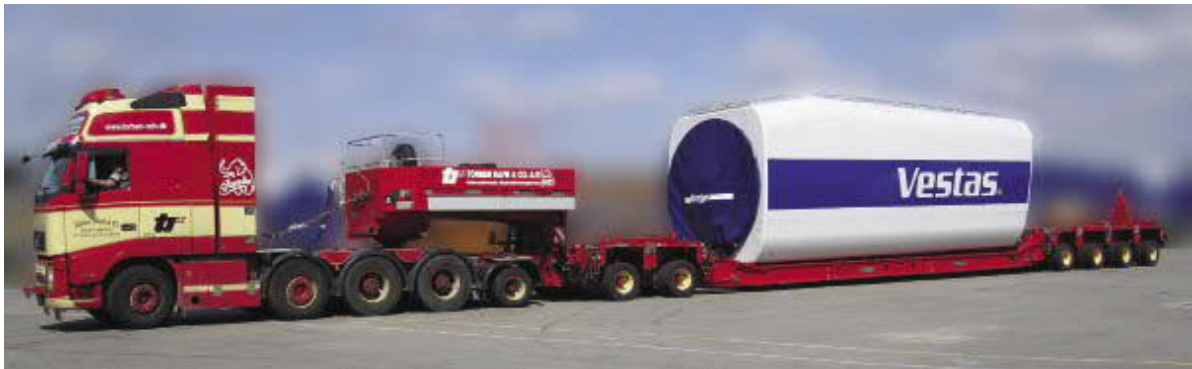
Figure 4-3: Transporting the Nacelle (Dvorak, 2010)
