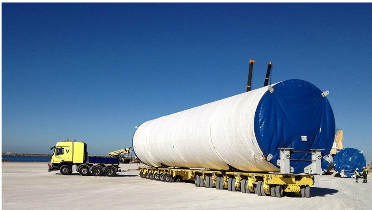
Figure 4-5: Transporting the Tower Sections (Montiea, 2014)
