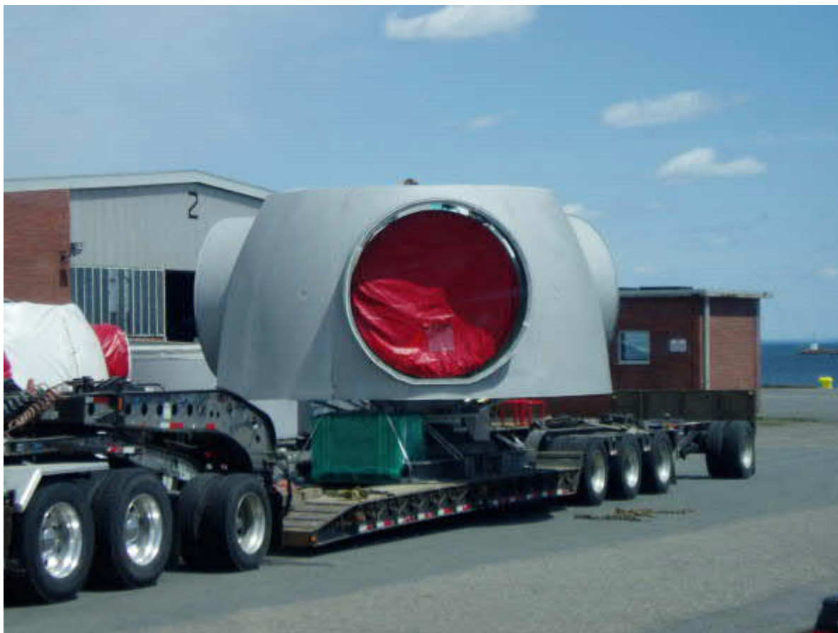
Figure 4-6: Transporting the rotor hub (Richardstransport, n.d.)
