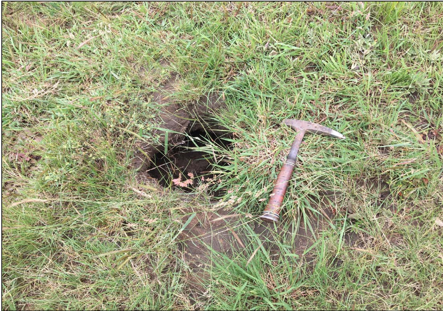
SOIL PIPING ADJACENT TO TRIAL HOLE D
