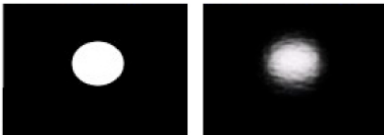
Figure 10: Reflection Characteristics of normal glass (left) and PV glass (right)
