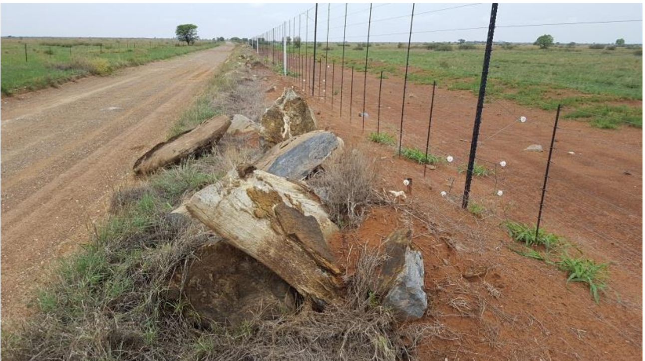
Figure 8. View from the area of hard, shallow underlying dolomite rock that has been excavated during the planting of fence poles. Such rock appears to underlie the whole site, either with secondary limestone formation above it (Figure 7), or not.
