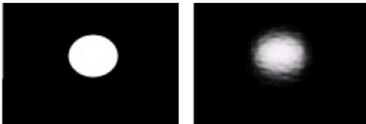
Figure 10: Reflection Characteristics of normal glass (left) and PV glass (right)
