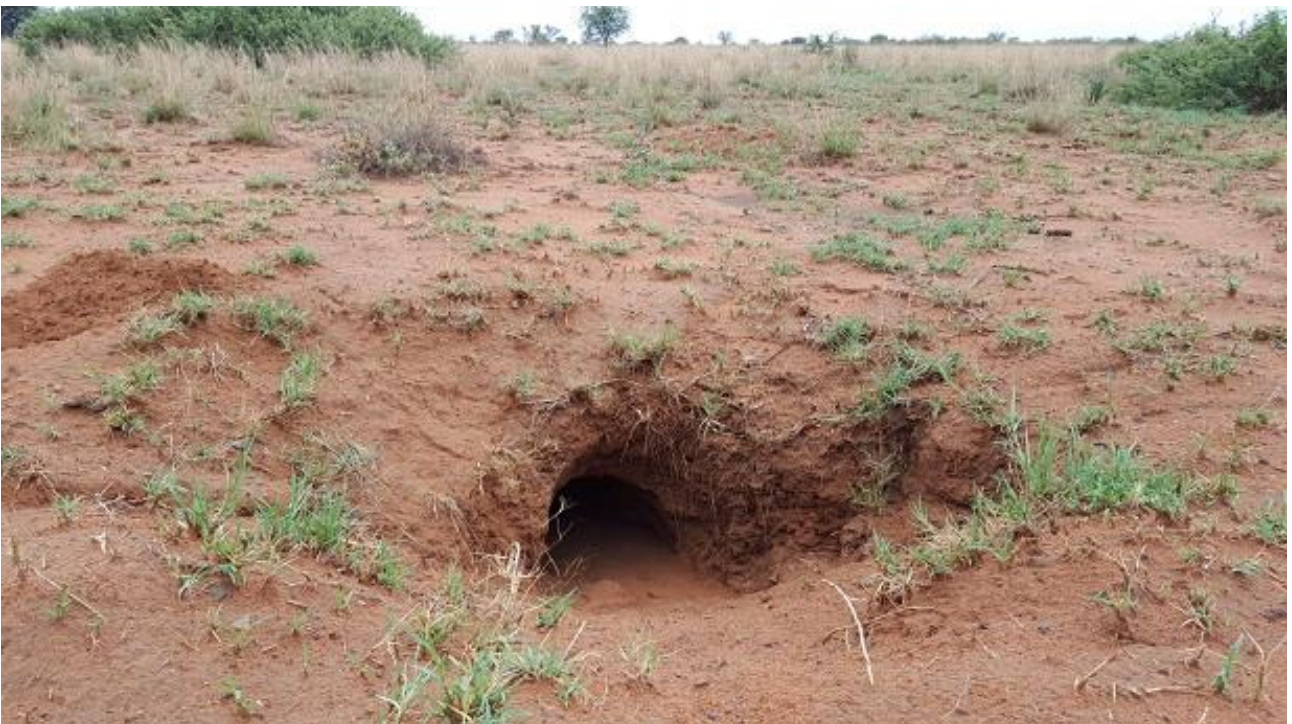
Figure 5. View of typical soil conditions on site (Clovelly soil form), as exposed in aardvark burrow.
