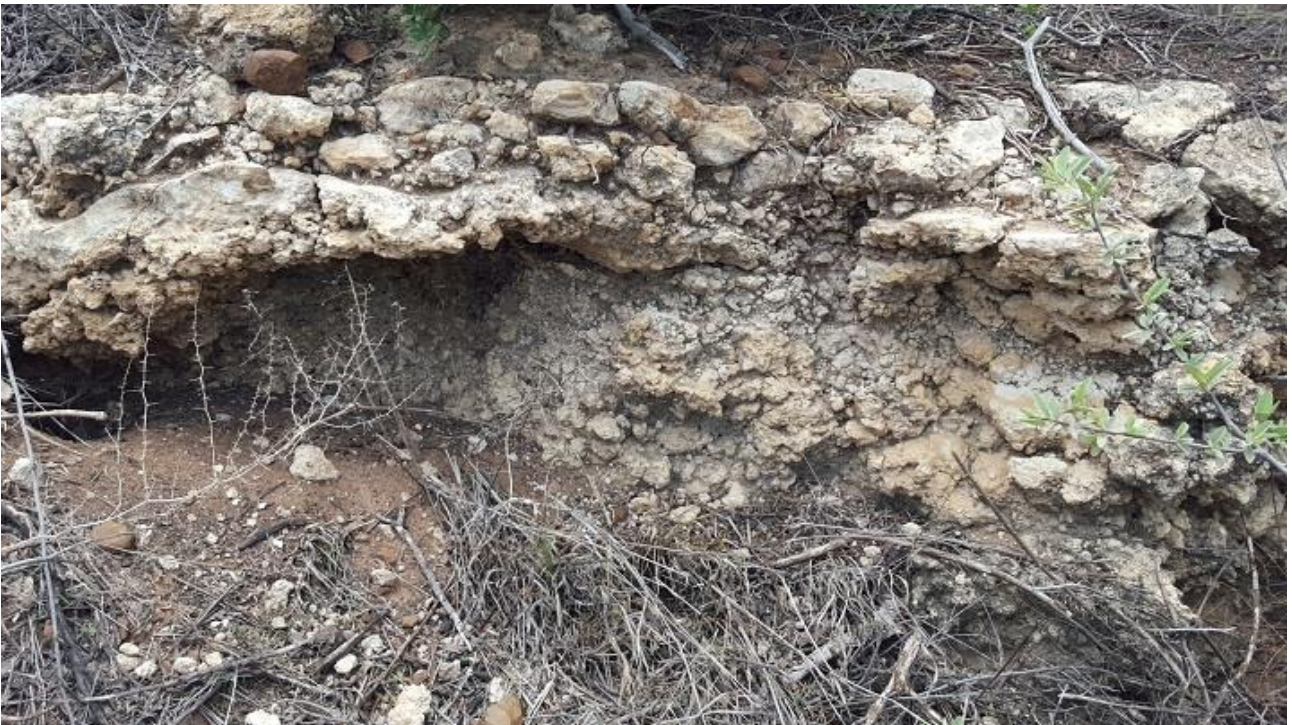
Figure 5. Photo of typical, shallow soil profile of the Coega soil form exposed in excavation along the road on the boundary of the site (sample point 1).
