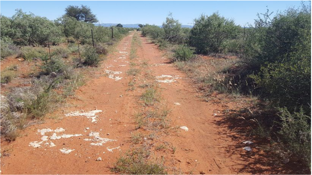
Figure 5. View of typical conditions across the site. Note the hardpan carbonate occurring at the soil surface.
