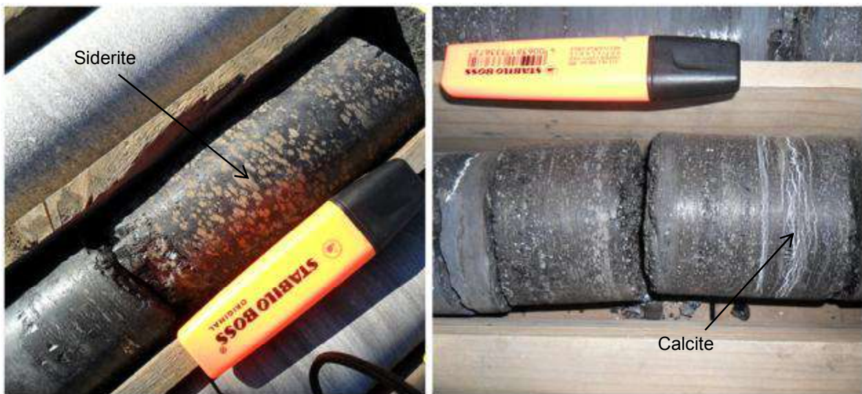
Figure 7: Siderite nodules (brown spots) and calcite (white veins) in coal.
