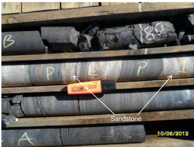
Figure 9: Channel sandstone parting (PLP1)
