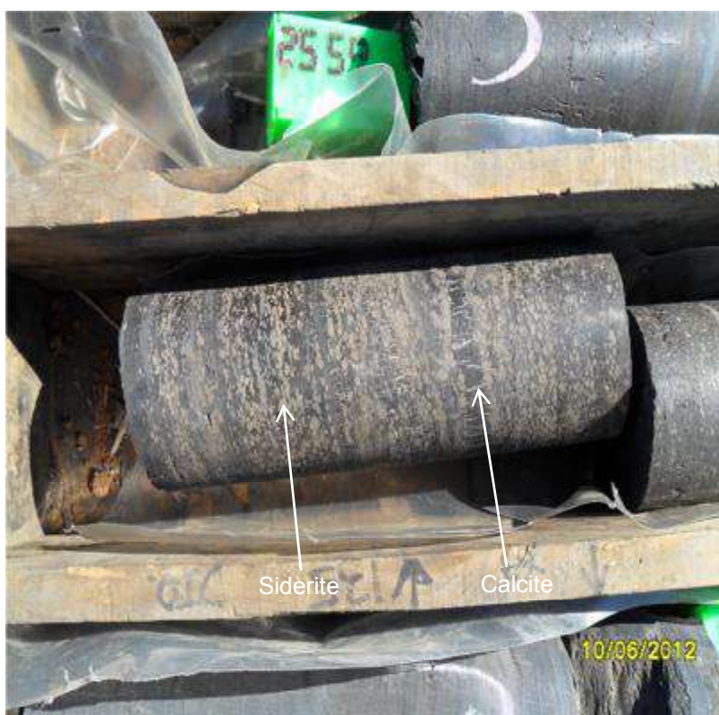
Figure 11: Calcite and siderite in Upper Ecca coal ply
