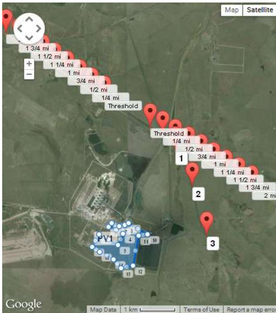
Figure 7, Location of the array and possible sensitive receivers input into the glare model
